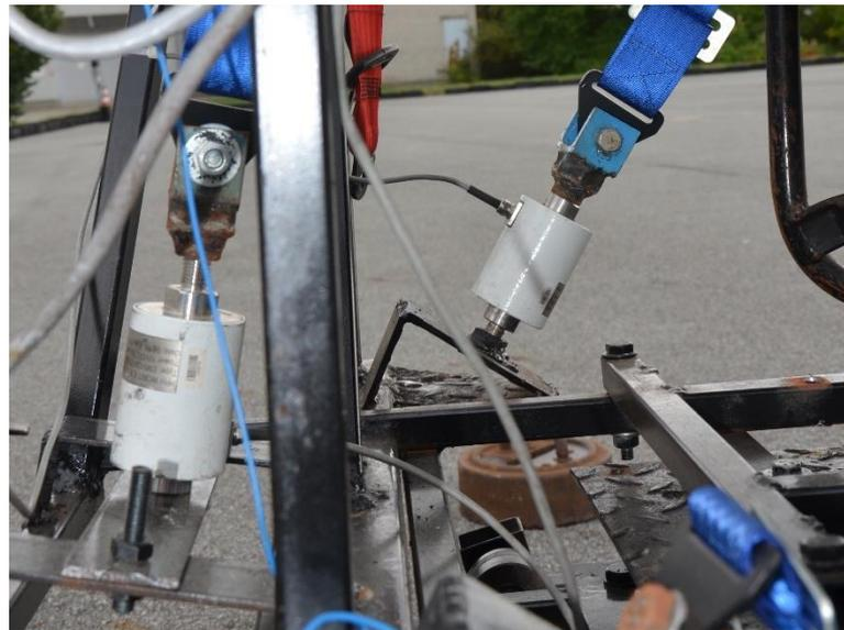
**Figure 2.** Force sensors in seat belts EMS 150.
