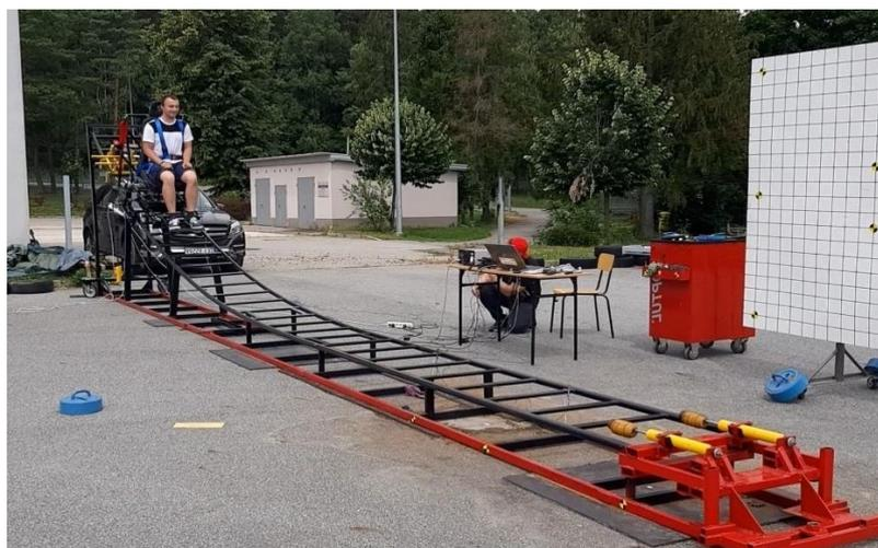
**Figure 1.** Test bench for low-speed crash tests.
