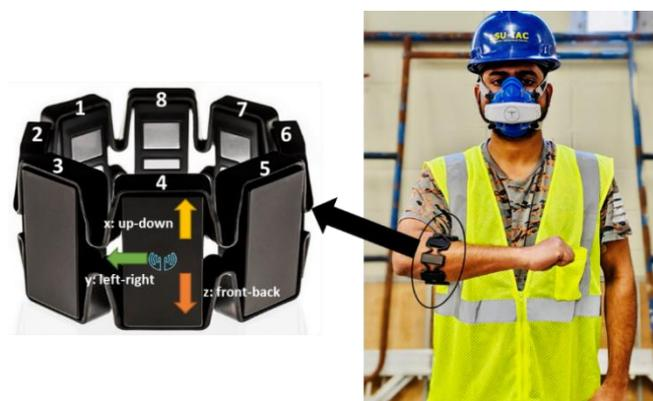
**Figure 5.** A participant wearing a forearm Myo armband and metabolic analyzer.
