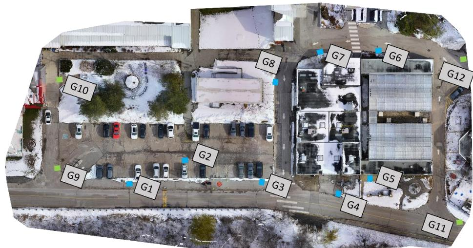
**Figure 4.** Ground control points (GCPs) and checkpoints distribution in study area.
