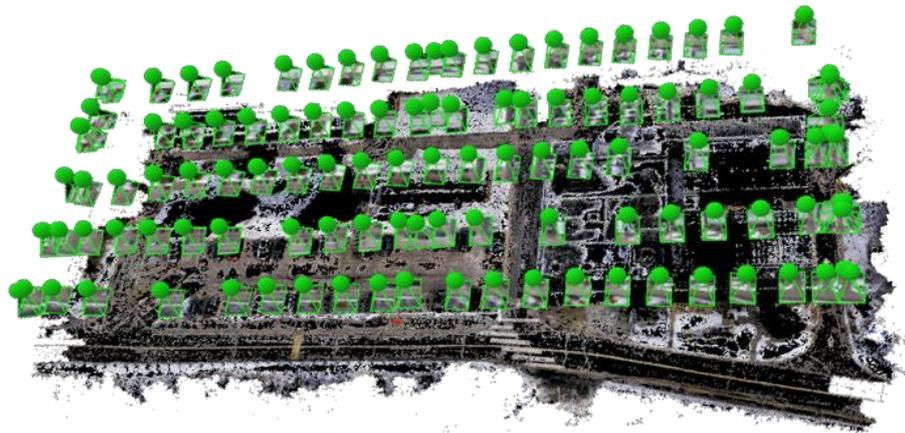
**Figure 5.** Camera poses estimated using Pix4D mapper software.
