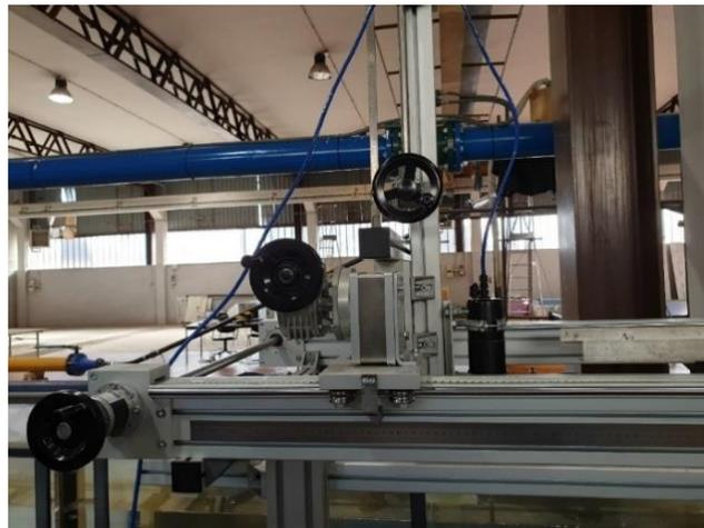
Figure 4. 3D instrument moving system of graduation scales.
