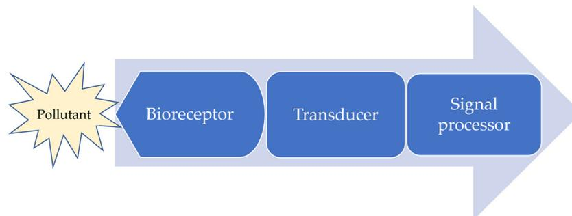
**Figure 1.** Operation of a biosensor.
