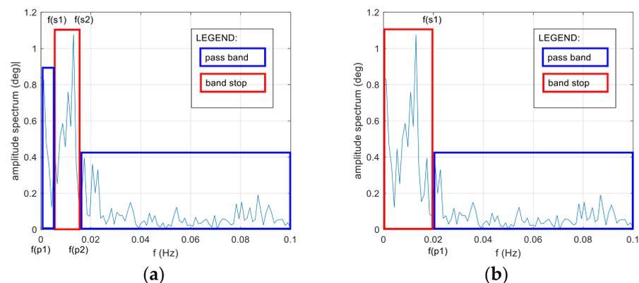
**Figure 1.** General model oscillation, dynamic conditions. (a) Stop band of 0.005–0.015 Hz. (b) Pass band of 0.02 Hz.  $f(p)$ —frequency pass band,  $f(s)$ —frequency stop band.
