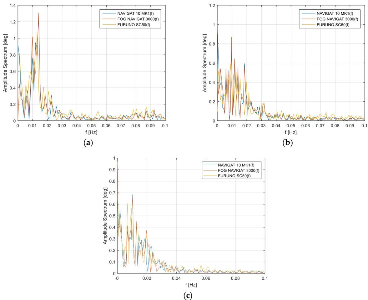
**Figure 4.** One-sided amplitude spectrum of the heading errors in the frequency domain: (a) Test #1, (b) Test #2, (c) Test #3.
