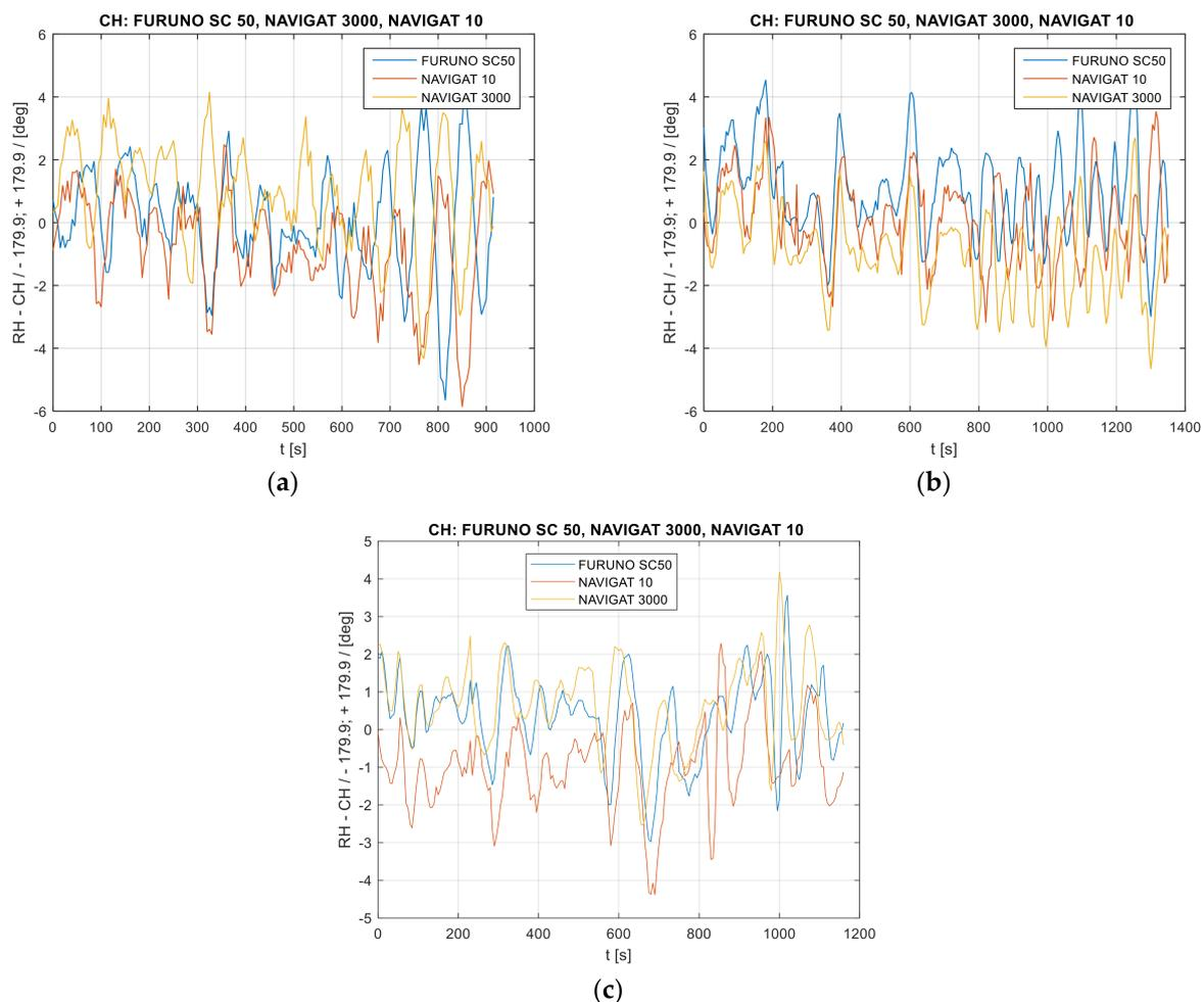
**Figure 3.** Heading recordings: (a) Test #1, (b) Test #2, (c) Test #3. The heading error amplitude distribution in the time domain. The heading values were reduced by the mean measurement from three heading systems.
