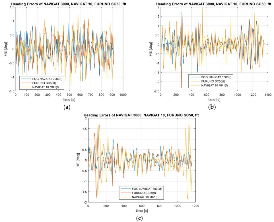
**Figure 6.** Absolute errors of the FOG 3000, FURUNO SC50, and NAVIGAT X MK1 compass heading after the application of the FIR filter with a pass-band of 0.02 Hz, (a) Test #1, (b) Test #2, (c) Test #3.
