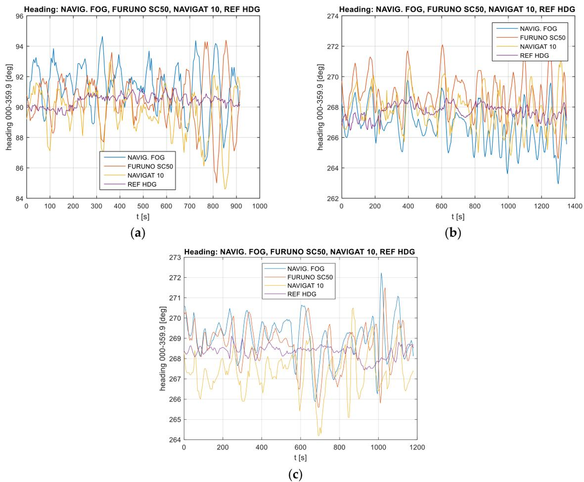
**Figure 2.** Heading recordings: (a) Test #1, (b) Test #2, (c) Test #3. The measurement was performed by the post-processing method.
