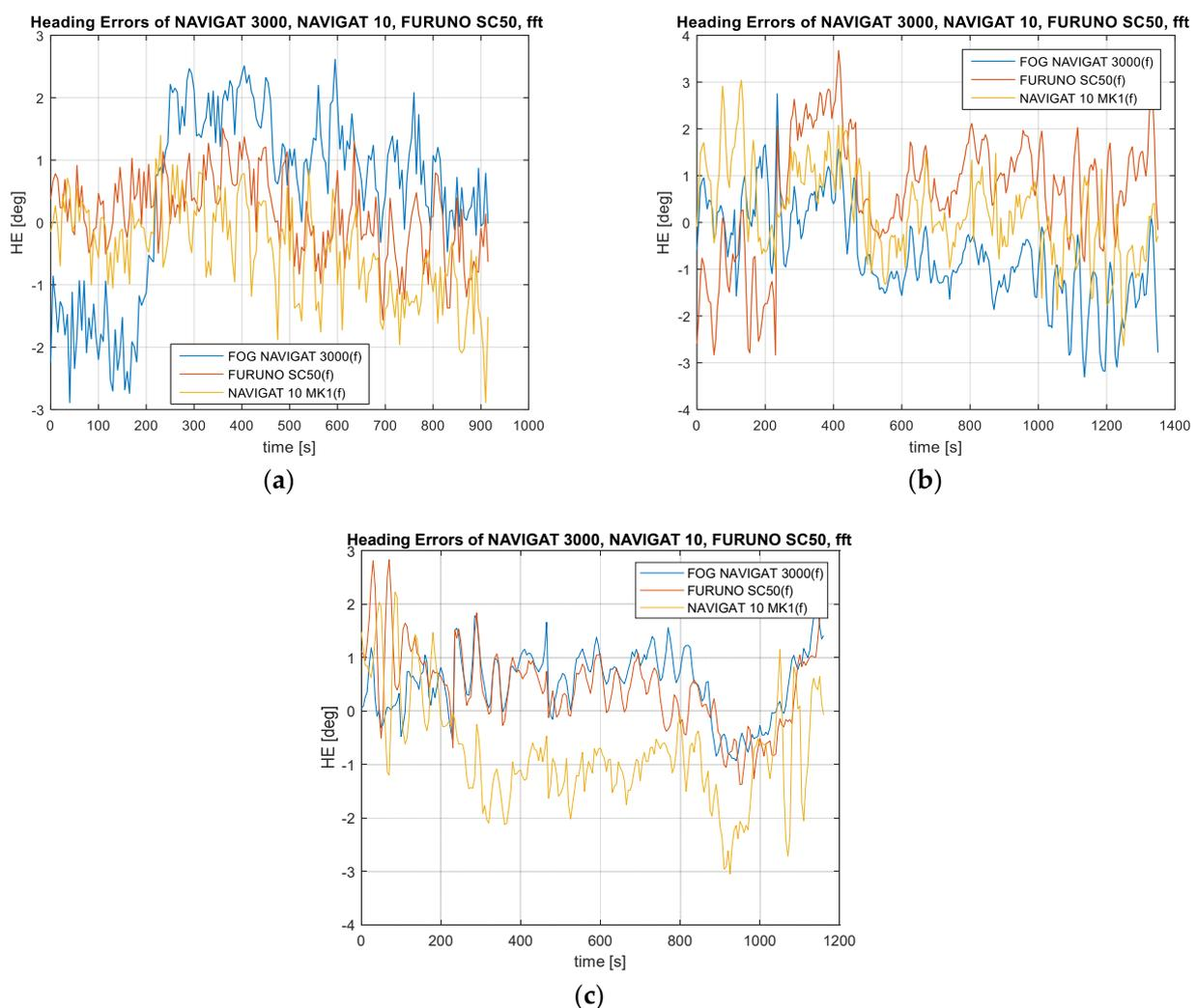
**Figure 5.** Heading amplitude error of the FOG 3000, FURUNO SC50, and NAVIGAT 10 MK1 compass heading after the application of the FIR filter with a stop-band of 0.005–0.015 Hz, (a) Test #1, (b) Test #2, (c) Test #3.
