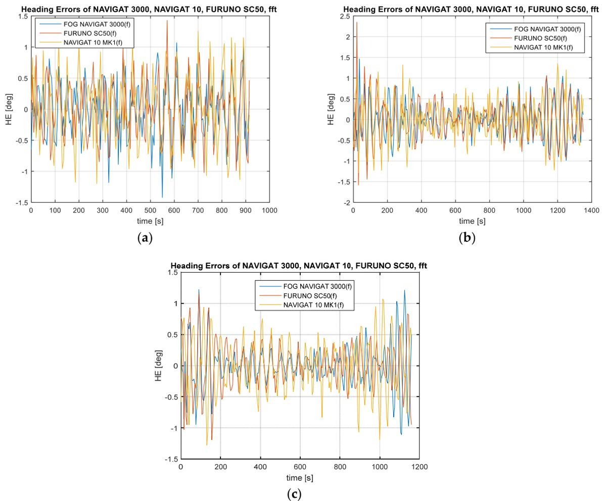
**Figure 8.** Absolute errors of the FOG 3000, FURUNO SC50, and NAVIGAT X MK1 compass heading after the application of the IIR filter with a pass-band of 0.02 Hz, (a) Test #1, (b) Test #2, (c) Test #3.
