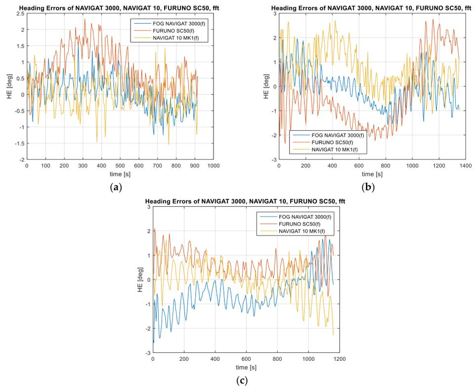
**Figure 7.** Absolute errors of the FOG 3000, FURUNO SC50, and NAVIGAT 10 MK1 compass heading after the application of the IIR filter with a stop-band of 0.005–0.015 Hz, (a) Test #1, (b) Test #2, (c) Test #3.
