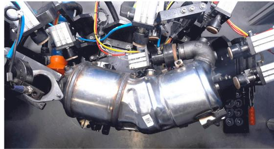
**Figure 2.** The assembled catalytic converter into the quality cell (courtesy of Marelli Europe SPA Green Technology Systems, Caivano, Italy).
