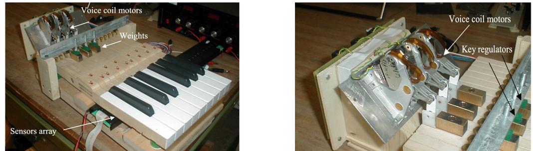
**Figure 8.** The Multi-Instrument active KEYboard (MIKEY) with a force feedback to the touch.
