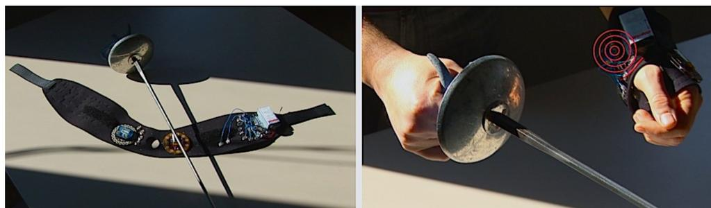
**Figure 17.** Glove with wrist strap for radio communication from the fencer to the scorekeeper and for actuator control.
