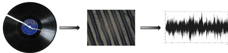
**Figure 12.** Photos of the GHOSTS system for reconstructing the audio signal from a still image of the surface of shellac discs.
