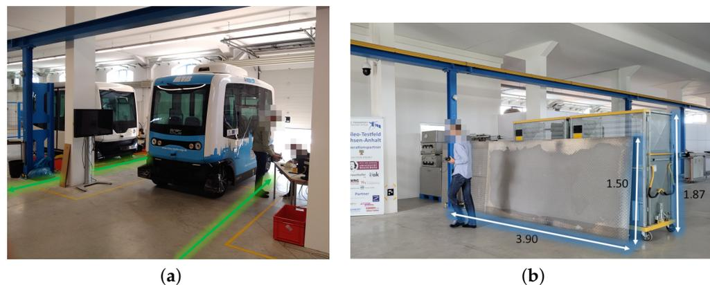
**Figure 7.** The objects used to obscure the line of sight in the Sparse NLOS environment: (a) start and end of test tracks with line of sight strongly obscured by vehicles and concrete pillars; (b) large metallic object in the center of the test environment.
