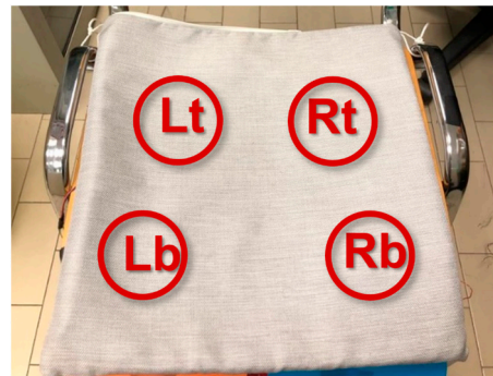
Figure 5. Pressure sensors' positioning into the cushion. The four sensors are identified by Lt ( Left-top ), Rt ( Right-top ), Lb ( Left-bottom ), Rb ( Right-bottom ).
