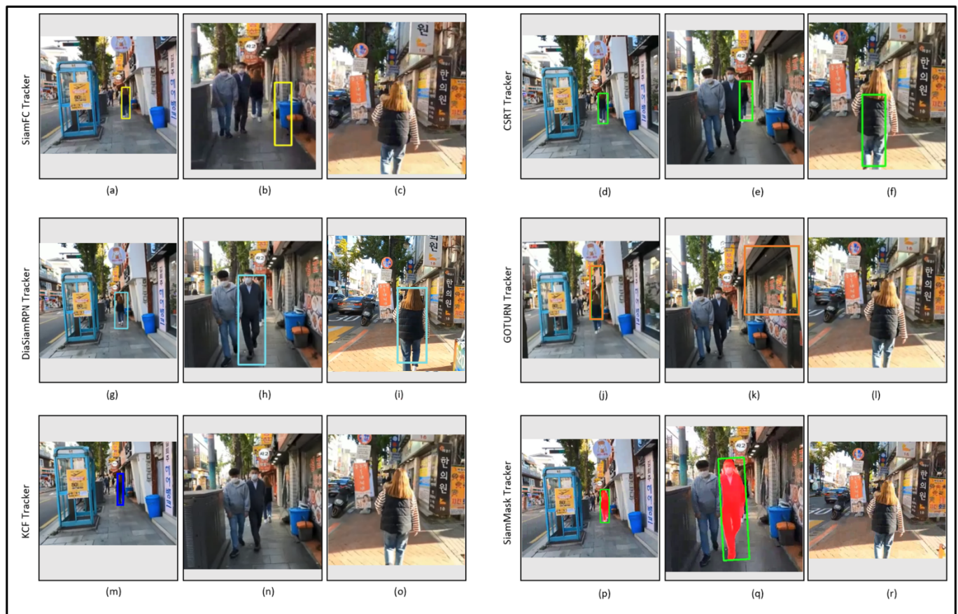
Figure 25. Outdoor video_4: Experimental results of the SiamFC, CSRT, DiaSiamRPN, GOTURN, KCF, and SiamMask trackers for the qualitative analysis.
