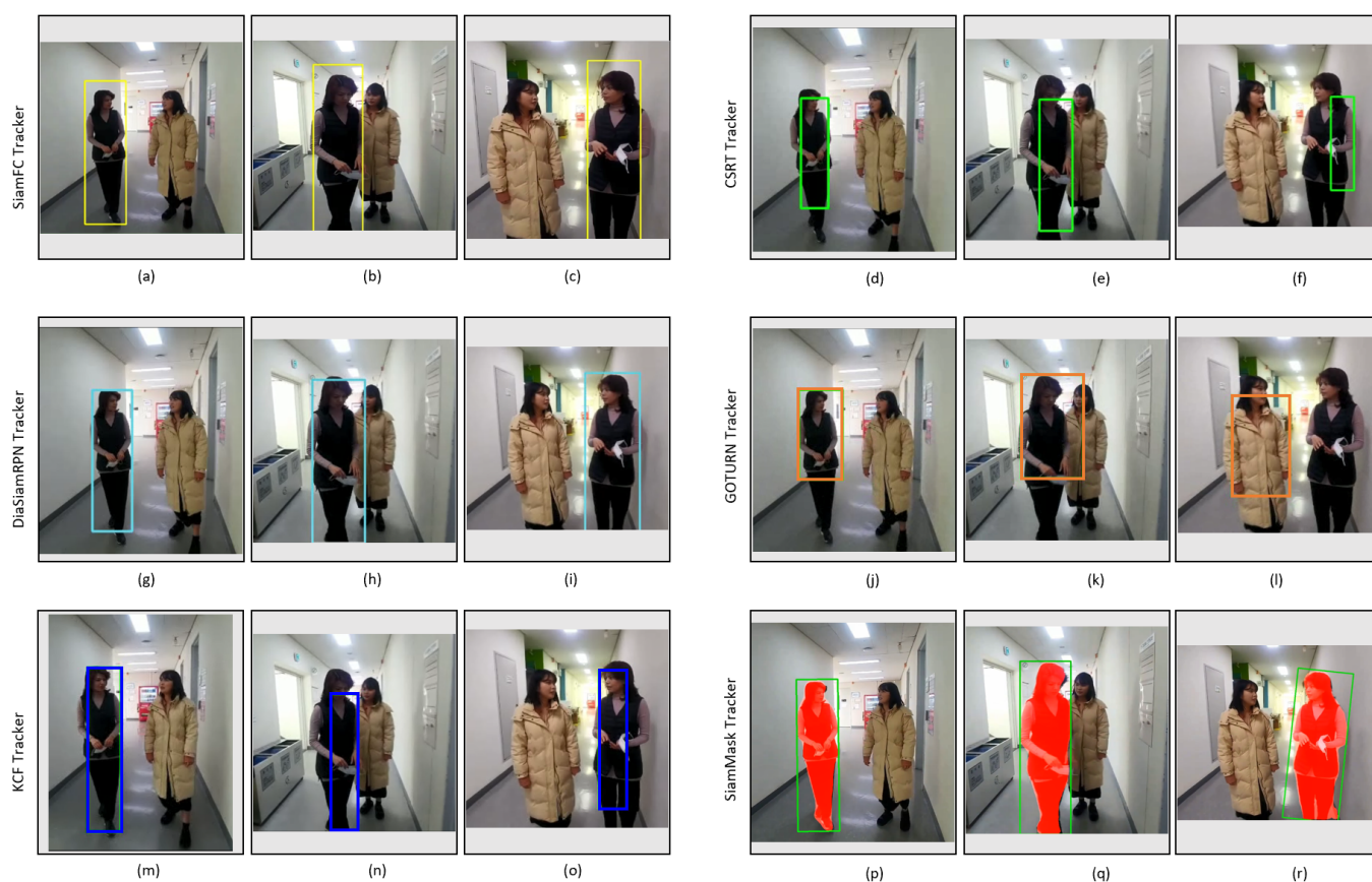
Figure 22. Indoor video_3: Experimental results of SiamFC, CSRT, DiaSiamRPN, GOTURN, KCF, and SiamMask trackers for qualitative analysis.
