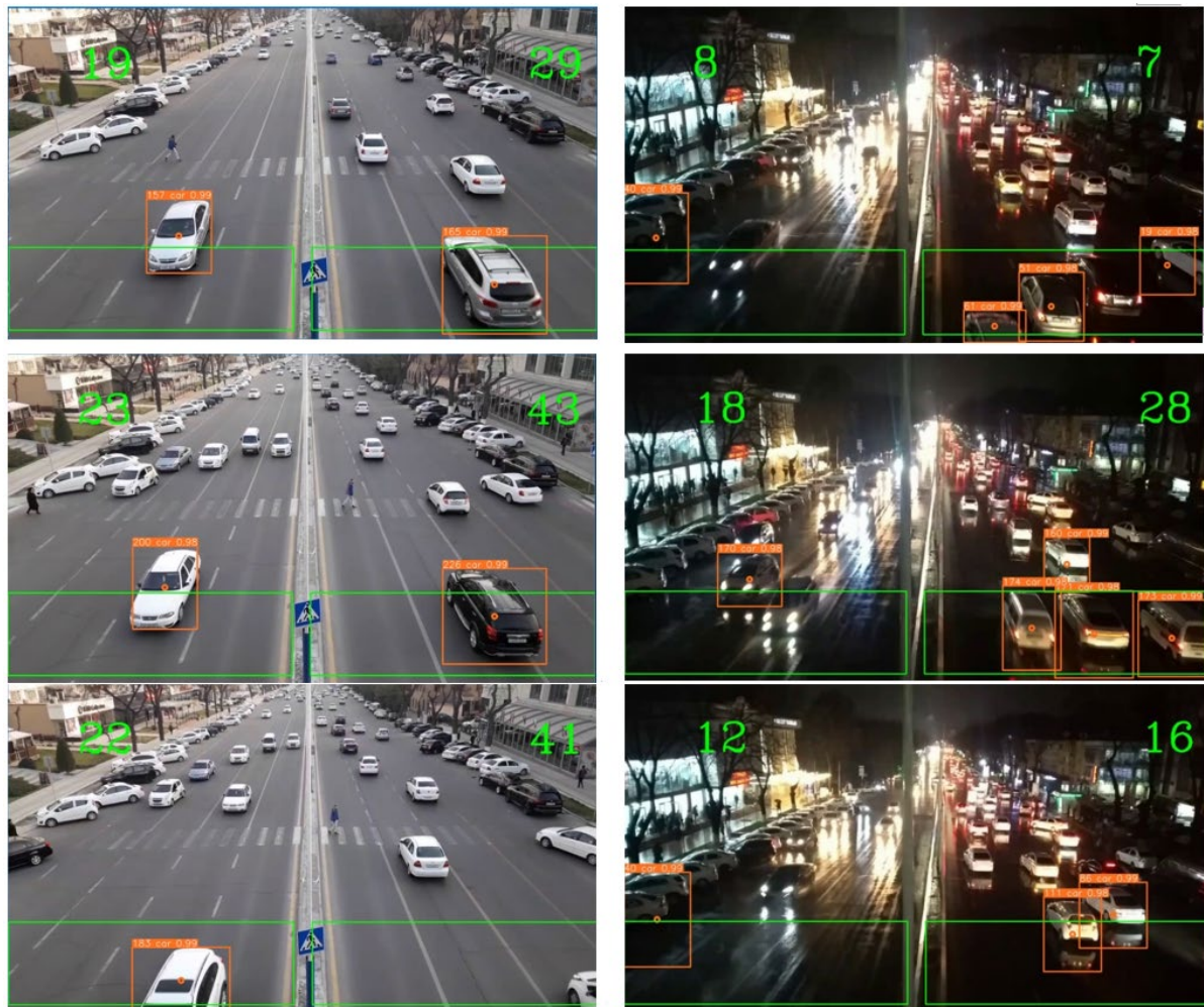
Figure 4. Examples of vehicle counting during daytime and nighttime.
