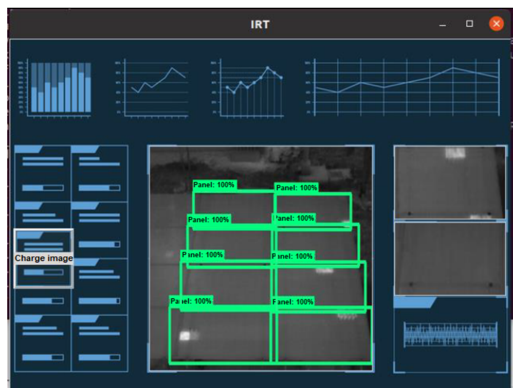
Figure 4. Graphical user interface for presentation of thermographic analysis and hot spot detection.
