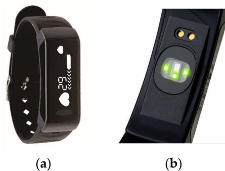
**Figure 2.** Wearable device for HRV measurement: (a) appearance on the front side; (b) three LEDs on the reverse side.
