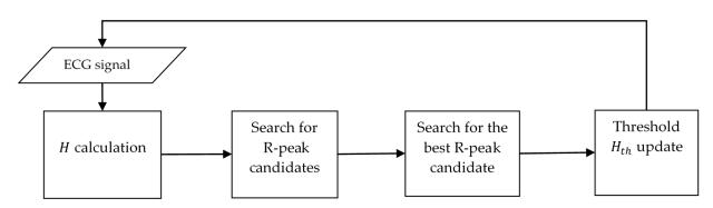
Figure 4. The proposed algorithm structure.
