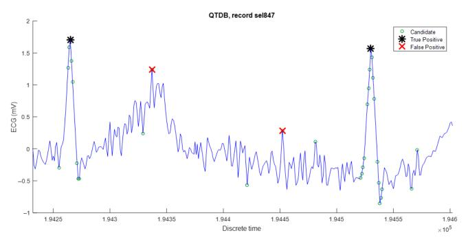
Figure 7. False positive R peaks provoked by high-frequency noise.
