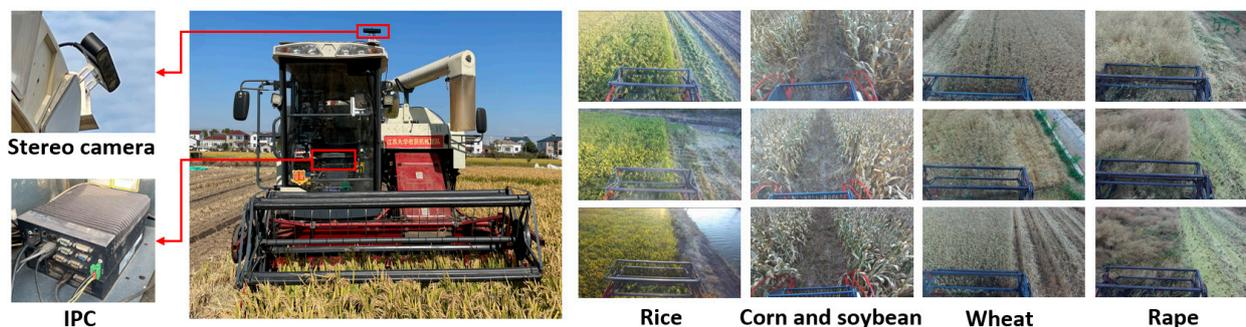
**Figure 2.** Camera and Industrial Personal Computer deployment, along with an example of the collected data.
