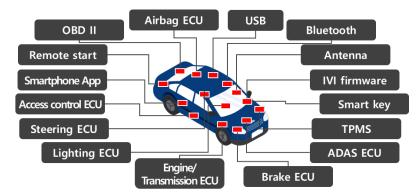
Figure 1. Connected car internal/external interfaces.
