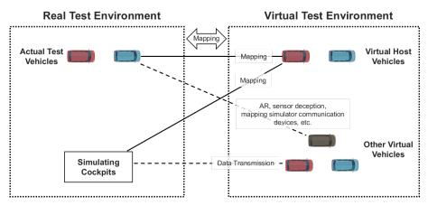
**Figure 6.** Environment configuration for parallel testing proposed by J. Wang et al. Application level security evaluation should be performed in an environment where a real device is mapped to a virtual test environment, as shown the actual test vehicle in this figure.
