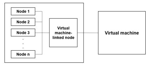
**Figure 7.** This figure shows the basic architecture of the virtual machine-based simulation node interoperation test environment configuration proposed in this paper. The user can configure the simulation nodes and the virtual machine as n:n according to the test situation.
