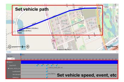
**Figure 9.** The simulation editor of the simulation equipment used in this paper. Using the scenario editor, the user can specify vehicle nodes' routes, speeds, and events. When the simulation is executed, each vehicle node drives according to the scenario specified by the user.
