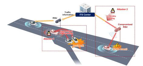
**Figure 5.** Examples of an attacks using V2X. Attacker 1 is the attacker's vehicle and causes an accident by sending a compromised BSM to near vehicles. Attacker 2 hacks the C-ITS infrastructure or RSU to send false information to the vehicle or force events, such as hard braking.
