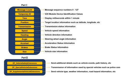
Figure 4. Structure of the BSM message Part I; Part II defined by SAE J2735.
