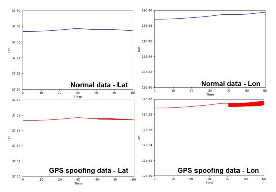
**Figure 12.** The graphs are the results of collecting and analyzing V2X messages generated in the simulation network after performing a GPS spoofing attack. With the occurrence time of V2X messages on the x-axis and the lat and lon values on the y-axis, the graphs show the changes when the GPS spoofing attack occurred. When driving normally, the values changed smoothly according to the driving route, but when the GPS spoofing occurred, the GPS value moved rapidly.
