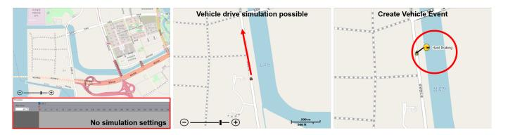
**Figure 10.** This figure shows driving by sending V2X data to a simulation node linked to the virtual machine and generating a vehicle event (hard braking) without using the scenario editor. The simulation node generates a message according to the standard specifications for the data received from the virtual machine and sends it to the simulation network. The user can create scenarios for specific situations or events according to the test cases.
