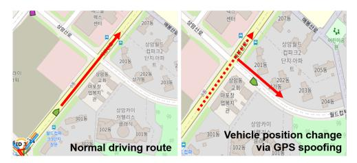
**Figure 11.** This figure shows a GPS spoofing scenario in which the GPS values are changed using the same address and ID in a vehicle node driving usually. The third vehicle perceives that the GPS information of the vehicle, with the pertinent ID, changes continuously, as shown in the figure.
