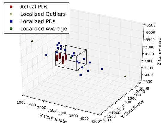
**Figure 11.** Localization results of multilateration on PD1 in KE20. The three axes are three dimensions of space (measured in mm).
