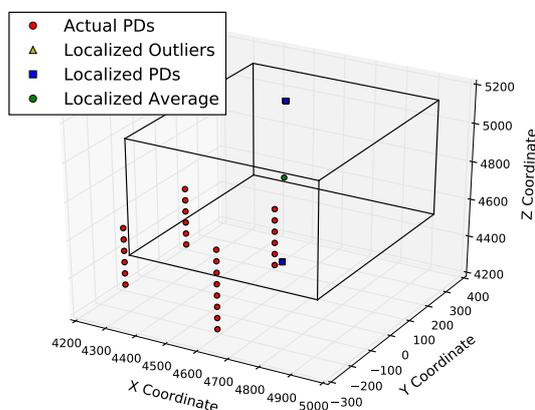
**Figure 14.** Localization results of CIFT are largely within 300 mm from the actual PD2 locations. The three axes are three dimensions of space (in mm).
