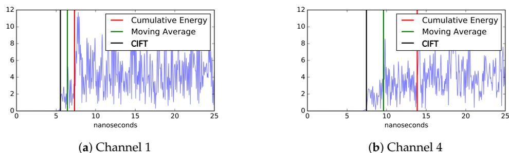
**Figure 10.** Signal arrival time of a simulated PD event in DL23. The horizontal axis is time and the vertical axis is the measured voltage (from FDTD simulation). In all cases, CIFT is able to identify the signal arrival time close to the known start time of 5 ns. In a low SNR case, shown in (b), the arrival time computed by the cumulative energy method is nearly 10 ns later than the actual signal start time, while the error of CIFT is only about 3 ns.
