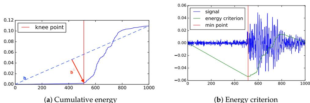
**Figure 2.** Two state-of-the-art timing methods. The horizontal axis is time steps and the vertical axis is energy (in  $V^2$ ).
