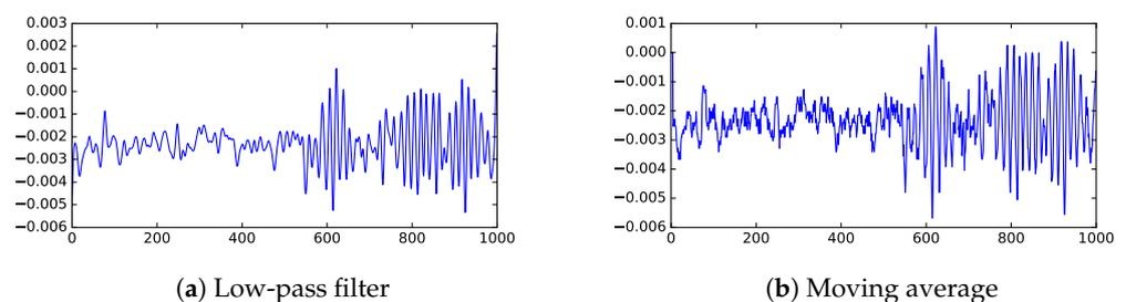
**Figure 4.** Filtered version of channel 4 data (low SNR). These two popular filtering techniques produce similar range of values. The horizontal axis is time steps (where each step is 0.4 ns) and the vertical axis shows UHF measurements processed with different techniques (in V).
