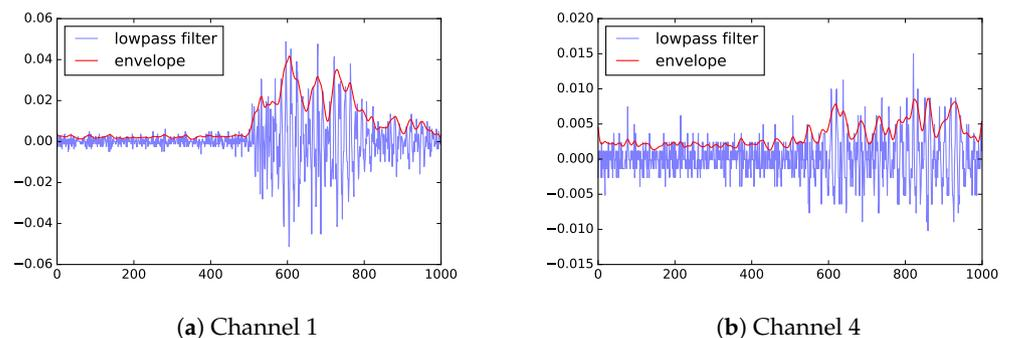
**Figure 5.** Envelope of two sample data sets. The horizontal axis is time steps (where each step is 0.4 ns) and the vertical axis shows UHF measurements (blue) along with envelope (red) (in V).
