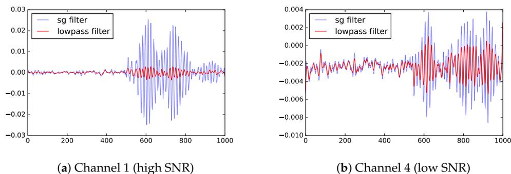
**Figure 6.** Savitzky–Golay (SG) filter works considerably better than low-pass filter. The horizontal axis is time steps (where each step is 0.4 ns) and the vertical axis shows UHF measurements processed with different techniques (in V).
