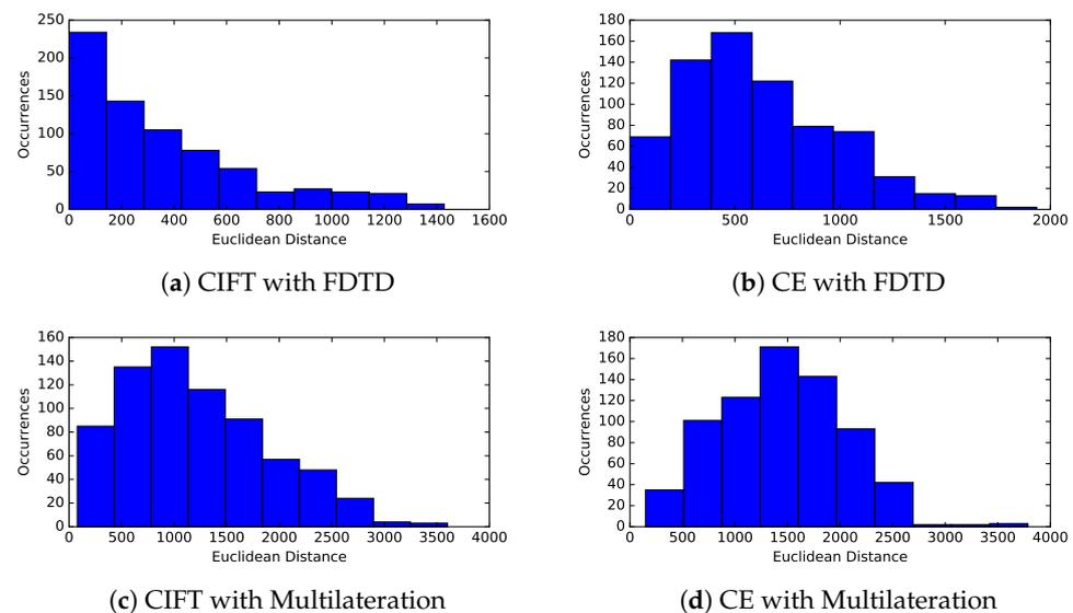
**Figure 15.** Error distribution (histogram) of PD events from DL23. The horizontal axis is the computed error. Each occurrence is from one simulated PD event from a FDTD cell. The average error using CIFT with FDTD is about 340 mm, which is close the FDTD mesh size of 300 mm and smaller than other methods tested. All methods have some cases with large errors that require further investigation.
