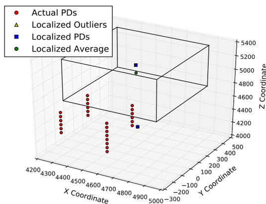
**Figure 13.** Localization results of cumulative energy are usually more than 300 mm away from the actual PD2 locations. The three axes are three dimensions of space (in mm).
