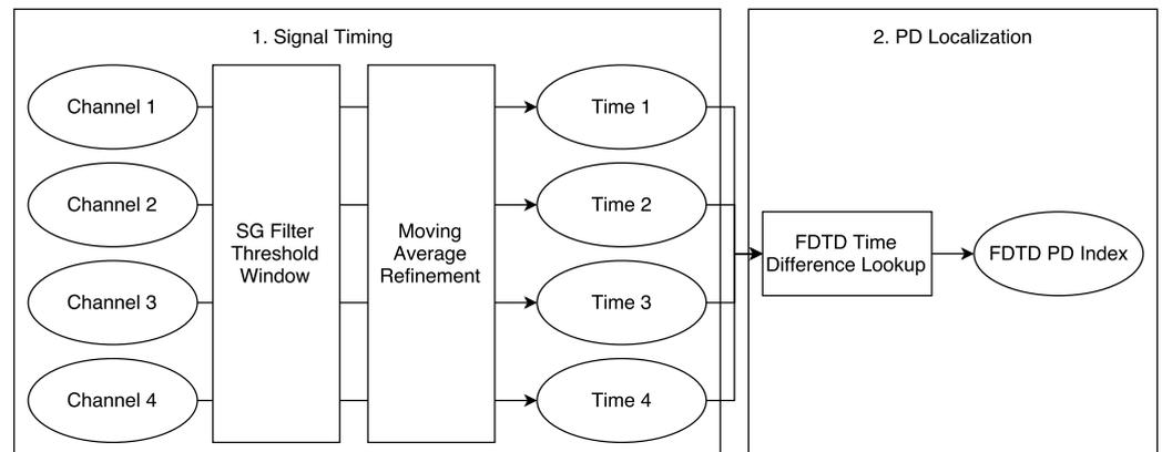
**Figure 8.** An overview of proposed PD localization procedure.
