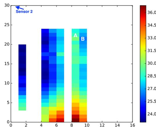
**Figure 7.** A heat map of arrival time to sensor 2 (located at the upper left corner) from a cross section of the FDTD mesh for KE20. The two axes are given in FDTD indices. Note that FDTD cell A is closer to sensor 2 than cell B, but the travel time from cell A is longer (green) than from cell B (blue).
