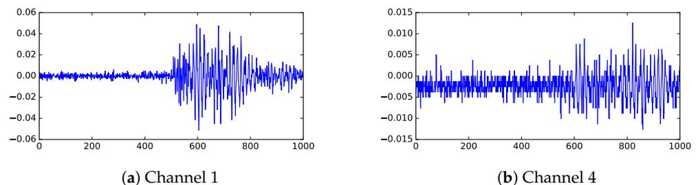
**Figure 1.** Sample raw data from UHF. The horizontal axis is time steps (where each step is 0.4 ns) and the vertical axis shows UHF measurements (in V).
