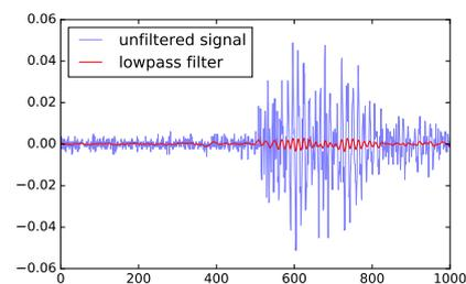
**Figure 3.** Low-pass filter could remove too much of the signal, an illustration with a series of high SNR (channel 1) data. The horizontal axis is time steps (where each step is 0.4 ns) and the vertical axis shows UHF measurements before and after filtering (in V).
