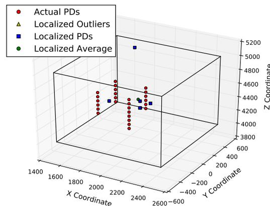
**Figure 12.** Localization results from FDTD table lookup on PD1 in KE20. The three axes are three dimensions of space (measured in mm). Many PD signals are determined to be from the same location, and there is no obvious outliers. All computed PD locations are well within the bounding box defined by the 500 mm tolerance.
