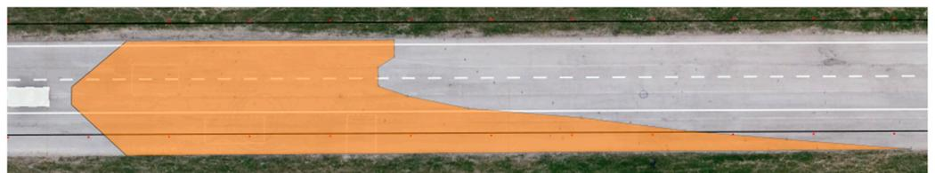
**Figure 31.** C 11.5 (I) class road—ankle-height illumination—Hyundai i40.
