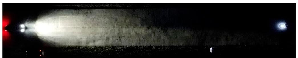
**Figure 8.** The illuminated person at a distance of 64.70 m from the Hyundai i40.
