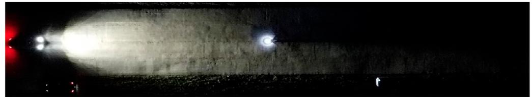
**Figure 6.** The illuminated person at a distance of 64.70 m from the Dacia Sandero.
