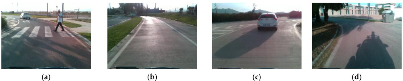
**Figure 2.** Images from dataset. (a) Pedestrian crossing; (b) saturation due to reflections on the road; (c) car braking; (d) complex shadows on the road.
