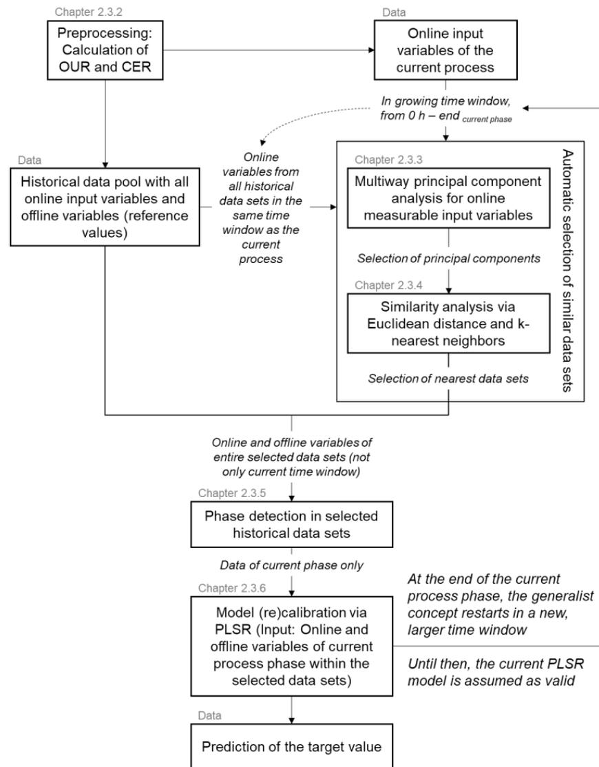
**Figure 1.** Structure of the generalist soft sensor concept. OUR = oxygen uptake rate; CER = carbon dioxide evolution rate; PLSR = partial least squares regression.
