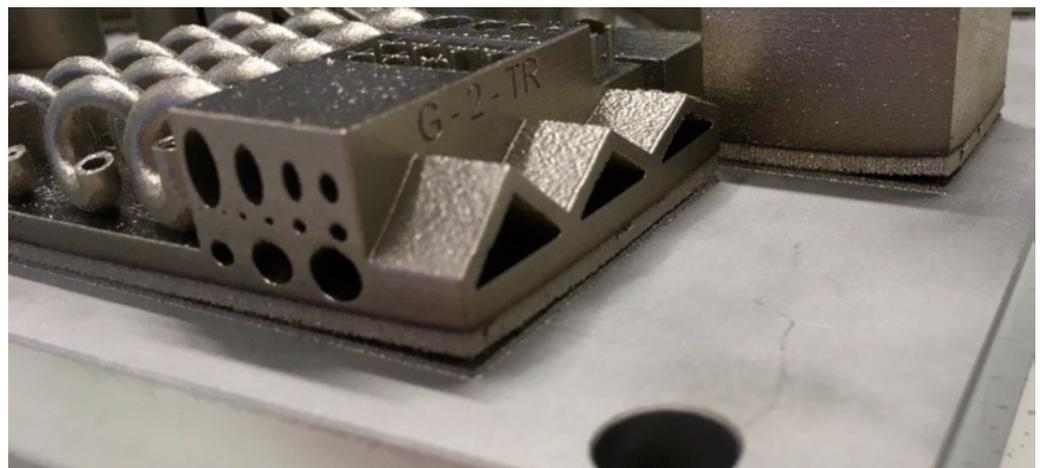
**Figure 7.** Example of layer delamination [30].
