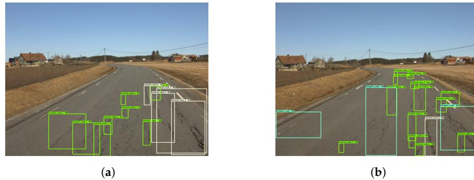
**Figure 10.** Cluttered detection—Model 2. The green and yellow boxes represent the vertical cracks while cyan colored boxes are the horizontal cracks.
