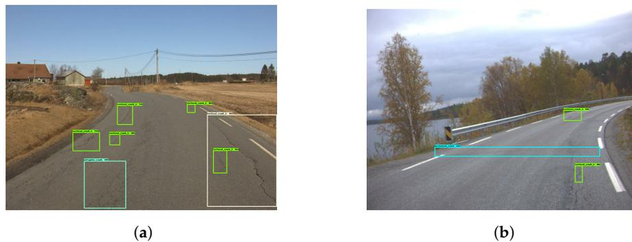
**Figure 13.** Low sensitivity in damage detection—Model 3. The green and yellow boxes represent the vertical cracks while cyan colored boxes are the horizontal cracks.
