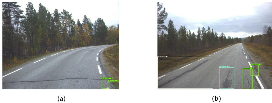
**Figure 16.** Missed damage detection—Model 4. The green and yellow boxes represent the vertical cracks while cyan colored boxes are the horizontal cracks.
