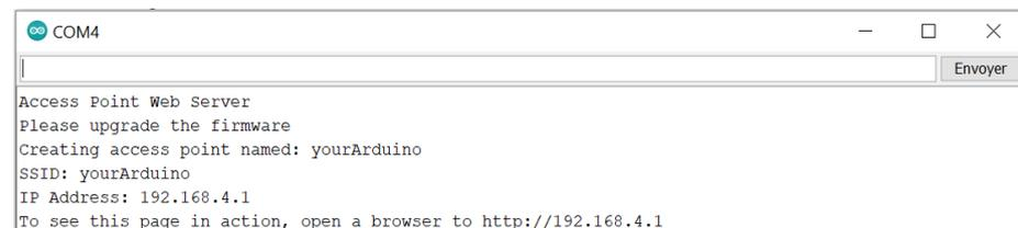
**Figure 13.** Arduino monitor showing the IP Address when creating the access point.
