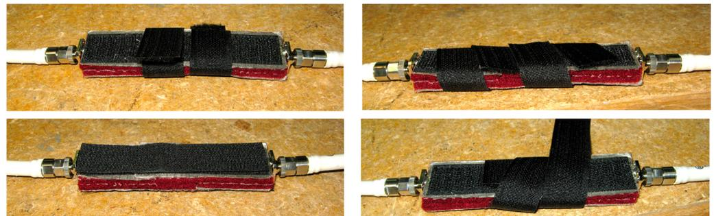
**Figure 14.** Non-conductive use of Velcro for interconnection of textile striplines in various ways of usage.
