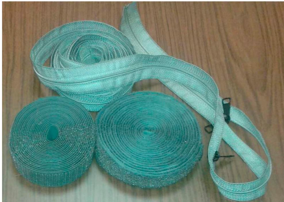
**Figure 9.** Conductive Velcro tape and Zip fastener from Shieldex, Bremen, Germany ([www.shieldex.de](http://www.shieldex.de), accessed on 2 March 2023).
