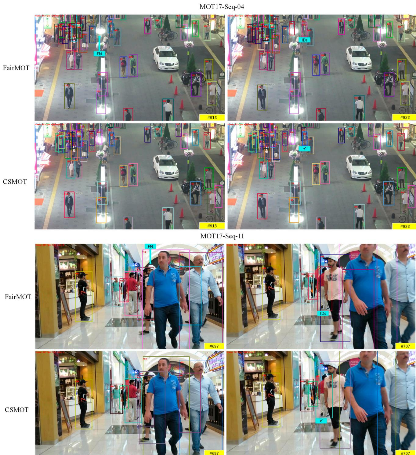
**Figure 5.** Robustness of our CSMOT compared to FairMOT. IDs and FN, respectively, indicate that the identity of the tracked object is switched and the object is not recognized. The checkmark indicates that the identity of the object is not switched.
