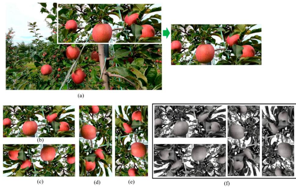
**Figure 3.** Dataset preparation and augmentation: (a) original RGB image, (b) cropped image from original image, (c) image rotated 180°, (d) image rotated 90° clockwise, (e) image rotated 90° counter-clockwise, and (f) all images when converted to grayscale.
