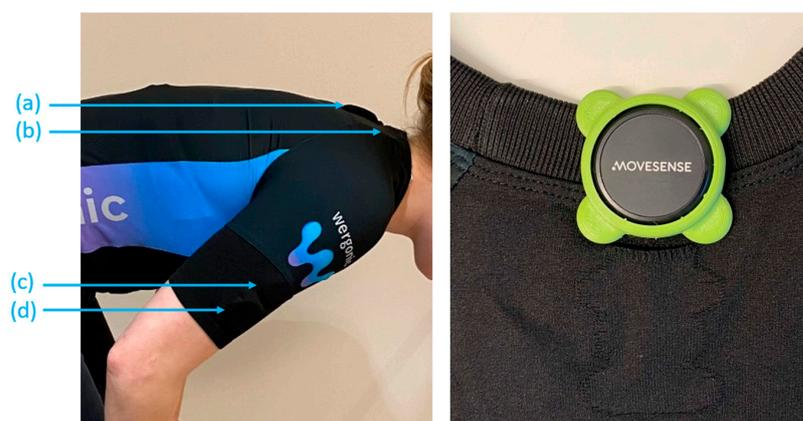
**Figure 1.** To the left: the two sensor setups showing (a) the trunk sensor in the shirt; (b) the trunk sensor on the skin; (c) the right upper arm sensor on the skin; and (d) the right upper arm sensor in the shirt. To the right: the Wergonic T-shirt pocket and the matching sensor case.
