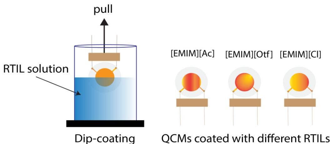
Figure 5. The dip-coating method for QCMs.
