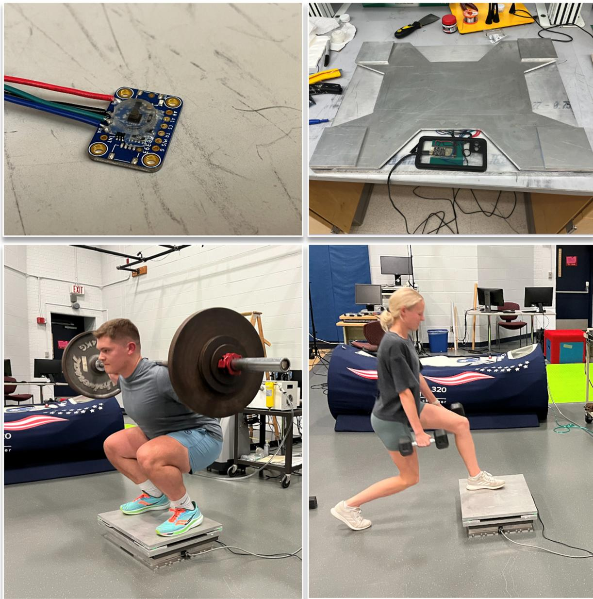
**Figure 1.** Images of a single sensor unit (top left), the assembled experimental force plate (top right), and participants performing weighted squats (bottom left) and lunges (bottom right) atop the Bertec (ground truth) force plate and the experimental force plate.
