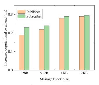
Figure 4. Increased computation overhead for encrypted transfers.
