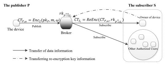
**Figure 2.** The framework of IoT end-to-end encryption system.
