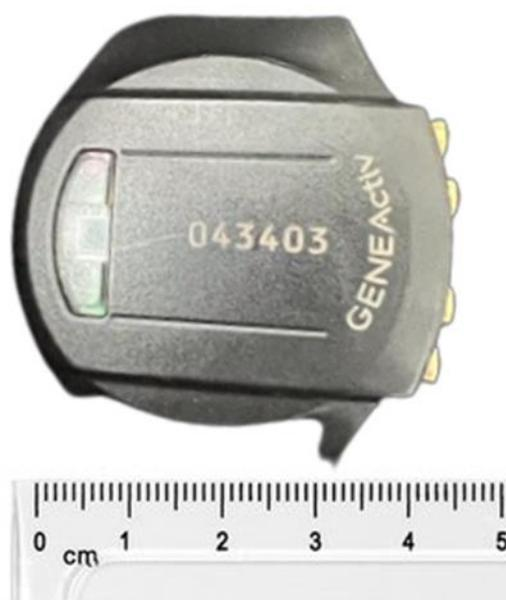
**Figure 3.** GENEActiv accelerometer (housing triaxial acceleration and temperature sensors).
