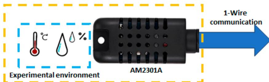
**Figure 9.** Architecture of the relative humidity and temperature sensor module.
