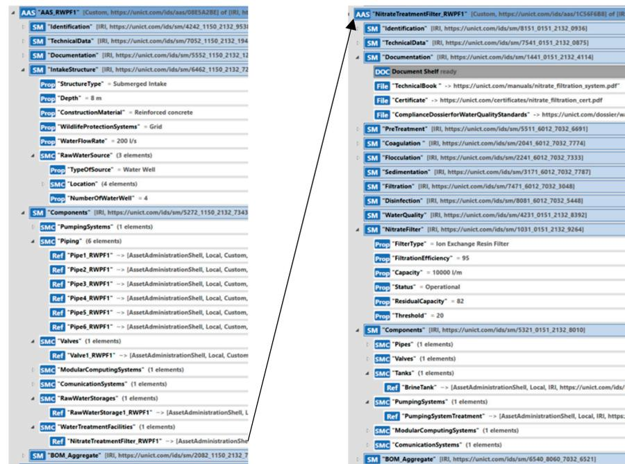
**Figure 18.** AAS instance of the AAS\_RWPF type modeling the RWPF1 including the nitrate treatment filter.
