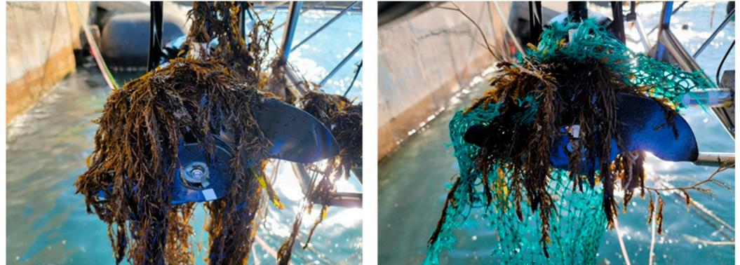
Figure 12. Naturally-occurred thruster entanglement faults during the experiment.
