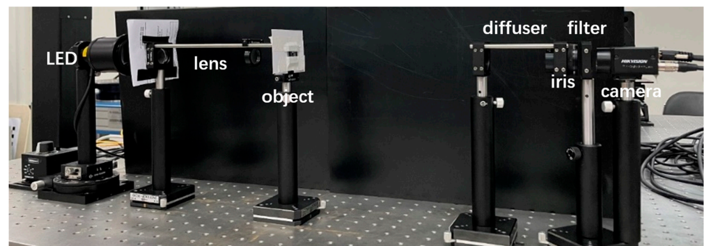
Figure 6. Physical diagram of the experimental light path.
