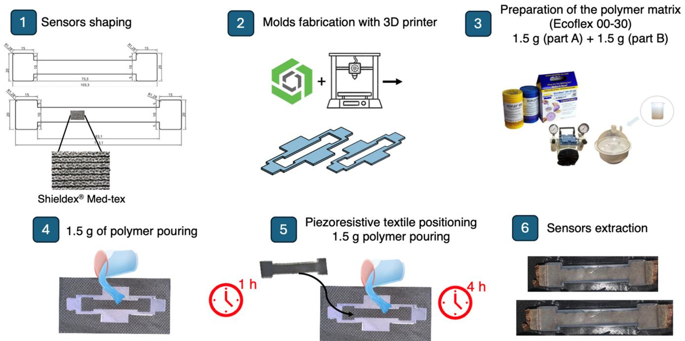
**Figure 3.** Schematization of the main steps carried out for the realization the two piezoresistive textile sensors and the integration into the wearable system by means of a polymer matrix.
