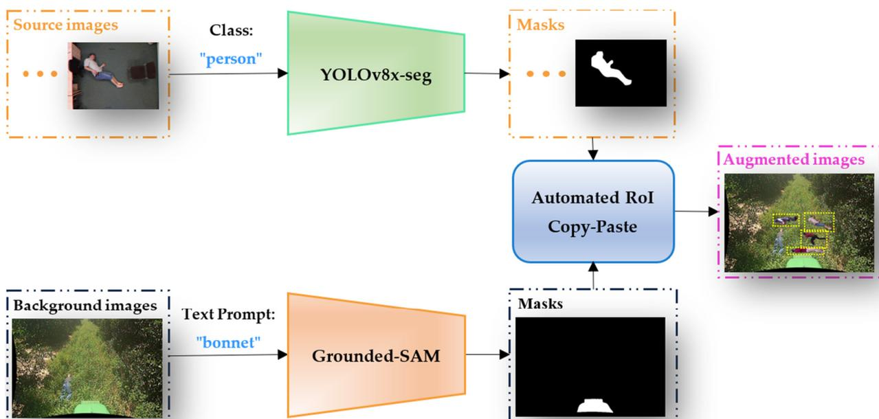
**Figure 2.** Framework of the ARCP pipeline. Objects with yellow dashed boxes in the augmented image represent objects pasted from the source images to the background image.
