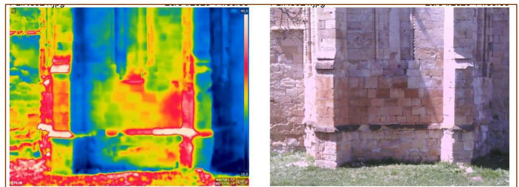
**Figure 9.** IR (left) and visible (right) images of the apse at local midday close to the Spring equinox.
