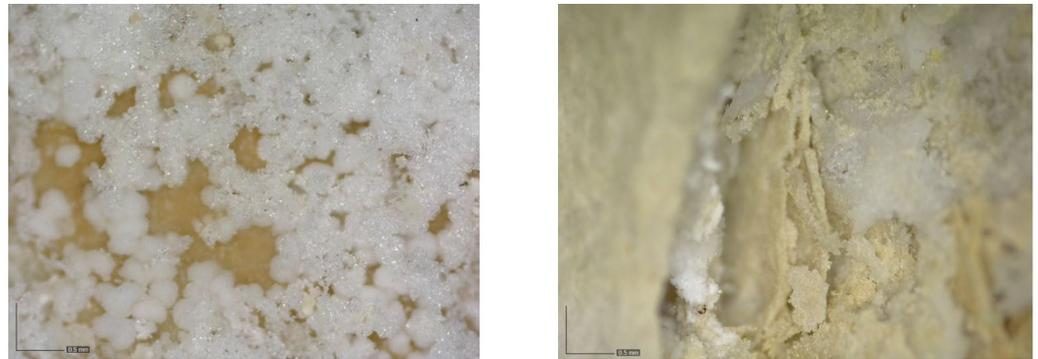
**Figure 10.** Photomicrographs obtained with a portable digital microscope showing powdery efflorescences (**left**) and subefflorescences associated with flacks and scales (**right**).
