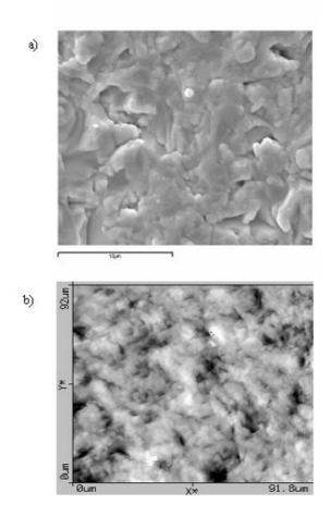
Figure 2. a) SEM image of WO<sub>3</sub> deposited via RF sputtering. b) AFM image of the same sample.
