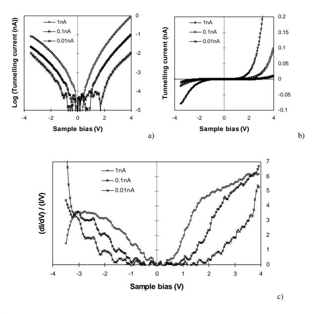
**Figure 5.** a) current versus sample bias curves acquired at three tip-sample separations. b) semi log plot of the three I(V) curves and c) (dI/dV)/(I/V) versus V spectra derived from the three I(V) curves. The high density of surface states induces an apparent reduction of surface band gap with respect to the bulk value.
