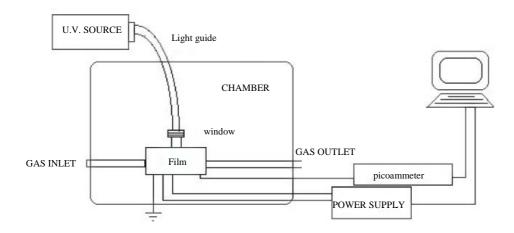
Figure 1. Experimental apparatus for photo-activation measurements.
