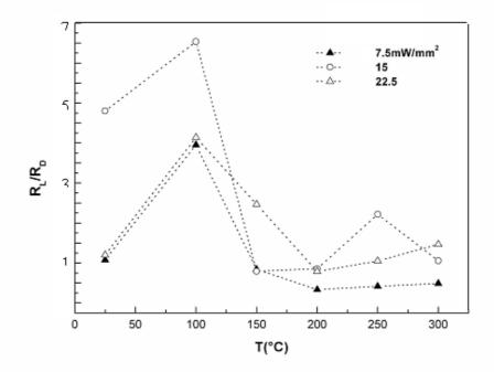
**Figure 8.** Ratio between the response ( $\Delta G/G$ ) toward 100 ppm of CO with light activation ( $R_L$ ) and in dark conditions ( $R_D$ ) as a function of the operating temperature and with different UV incident power. The best conditions for an increase in performance of the sensor are 100°C as operating temperature and 15 mW/mm<sup>2</sup> as incident UV power on the sensor.
