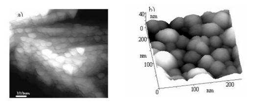
**Figure 3.** a) High resolution 1000x1000nm<sup>2</sup> contact AFM image acquired at a force setpoint of 20nN. The grey scale corresponds to a z-range of 140nm. b) 3D 250x250nm<sup>2</sup> constant current STM image acquired at a tip voltage of 3V and tunneling current setpoint of 0.6nA.
