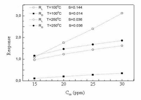
**Figure 7.** Response with light (15 mW/mm<sup>2</sup>) and in dark conditions as a function of CO concentration and sensitivity,  $S=\delta R/\delta C_{CO}$ .
