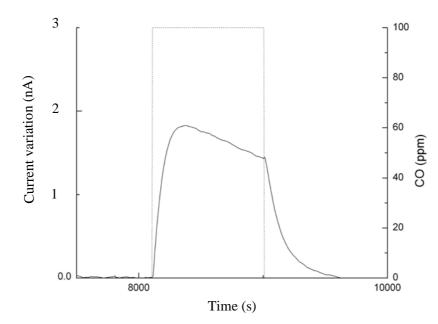
**Figure 6.** Dynamical response to a square pulse of 100 ppm of CO. Current rises up due to redox reactions at surface. The characteristic response time of a layer is visible.
