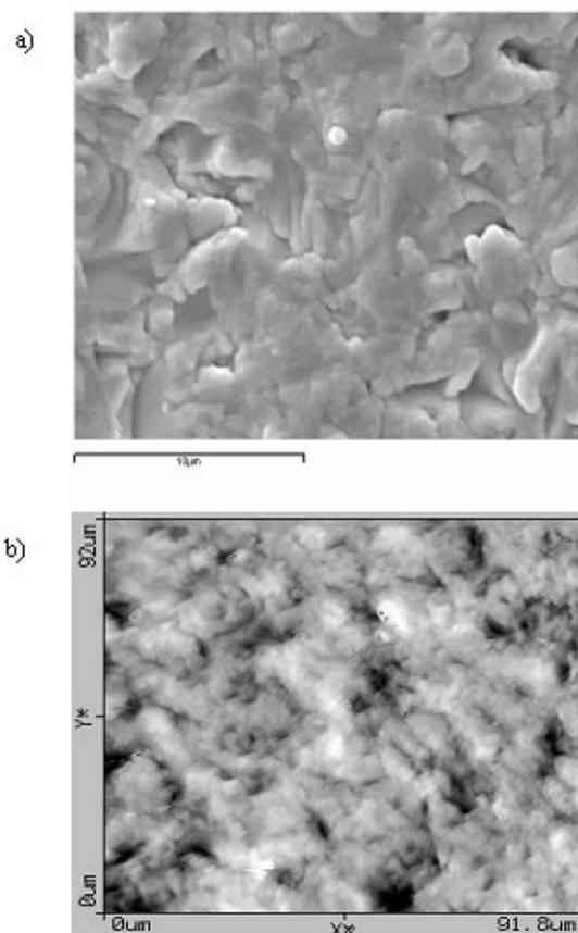
**Figure 2.** a) SEM image of  $\text{WO}_3$  deposited via RF sputtering. b) AFM image of the same sample.
