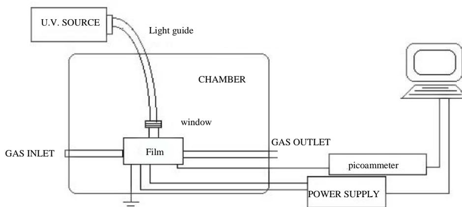
**Figure 1.** Experimental apparatus for photo-activation measurements.
