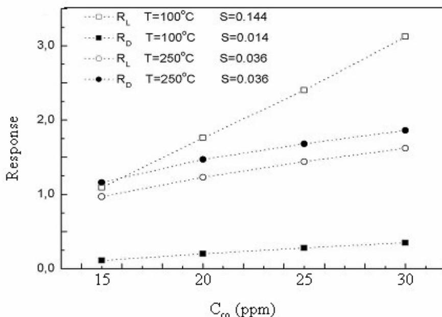
**Figure 7.** Response with light ( $15 \text{ mW/mm}^2$ ) and in dark conditions as a function of CO concentration and sensitivity,  $S = \delta R / \delta C_{CO}$ .
