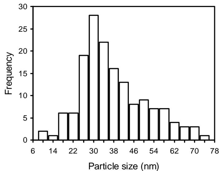
**Figure 4.** Particle size distribution extracted from STM images.
