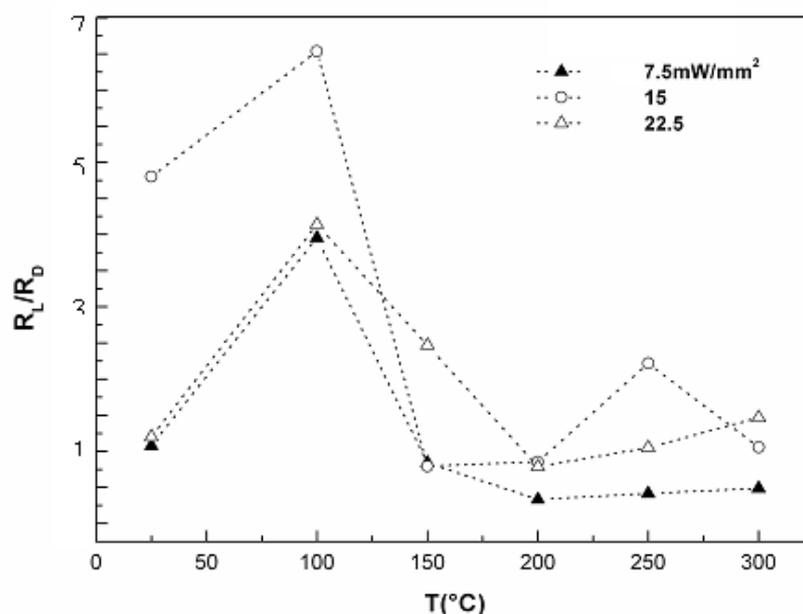
**Figure 8.** Ratio between the response ( $\Delta G/G$ ) toward 100 ppm of CO with light activation ( $R_L$ ) and in dark conditions ( $R_D$ ) as a function of the operating temperature and with different UV incident power. The best conditions for an increase in performance of the sensor are 100°C as operating temperature and 15 mW/mm<sup>2</sup> as incident UV power on the sensor.
