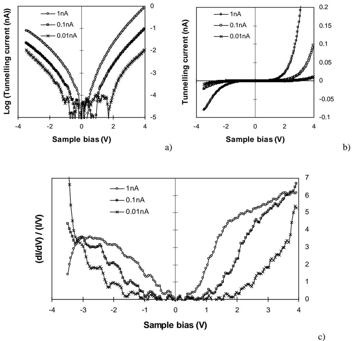
**Figure 5.** a) current versus sample bias curves acquired at three tip-sample separations. b) semi log plot of the three  $I(V)$  curves and c)  $(dI/dV)/(I/V)$  versus  $V$  spectra derived from the three  $I(V)$  curves. The high density of surface states induces an apparent reduction of surface band gap with respect to the bulk value.
