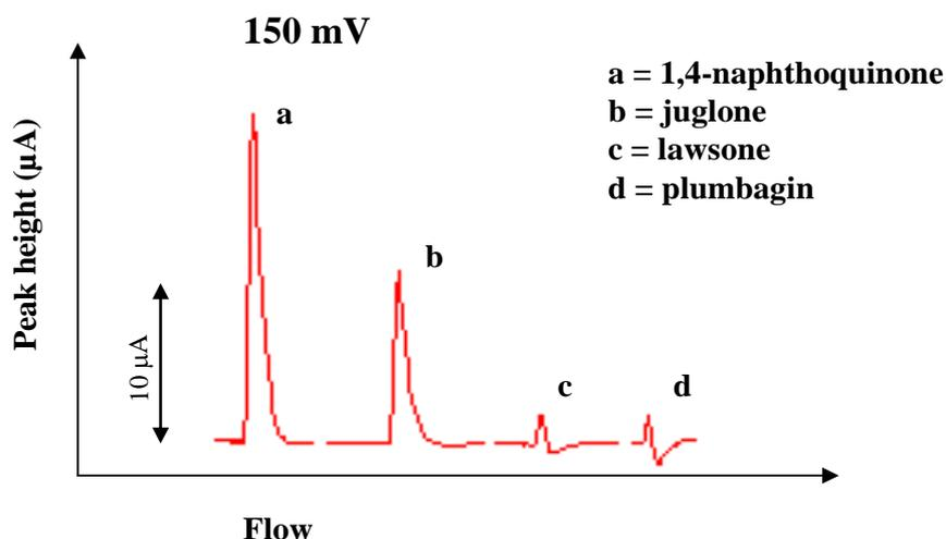
**Figure 5.** A FIA-amperometric record of the naphthoquinones ( $1 \mu\text{g}\cdot\text{ml}^{-1}$ ) at the potential of 150 mV. The flow rate of the electrolyte (0.2 M phosphate buffer, pH 5.5) was  $0.5 \text{ ml}\cdot\text{min}^{-1}$ . The sample ( $5 \mu\text{l}$ ) was injected manually. The working electrode was made from glassy carbon, auxiliary carbon electrode and referent hydrogen palladium electrode. For other details see “Materials and Methods” section.
