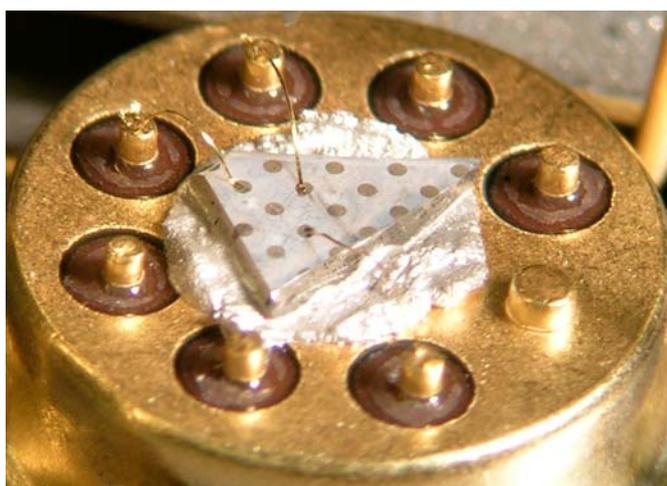
**Figure 9.** SEM of ZnO multiple nanorods (top) and photograph of the nanorods contacted by Al/Pt/Au electrodes (bottom). The ZnO chip has edge length  $\sim 5\text{ mm}$  in the bottom photo.
