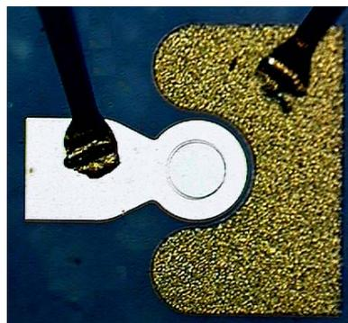
**Figure 2.** Cross-sectional schematic of completed MOS diode on AlGaN/GaN HEMT layer structure (top) and plan-view photograph of device (bottom).
