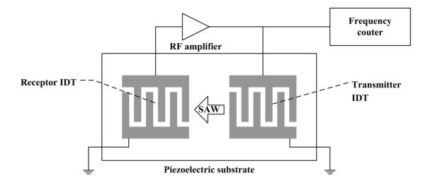
Figure 11. Configuration of surface acoustic wave sensor device.
