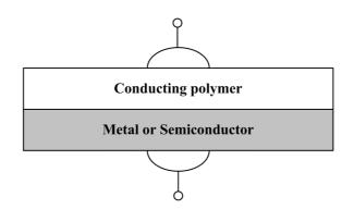
Figure 7. Configuration of diode device.
