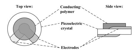
Figure 10. Configuration of quartz crystal microbalance sensor device.
