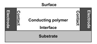
Figure 3. Configuration of chemresistor.
