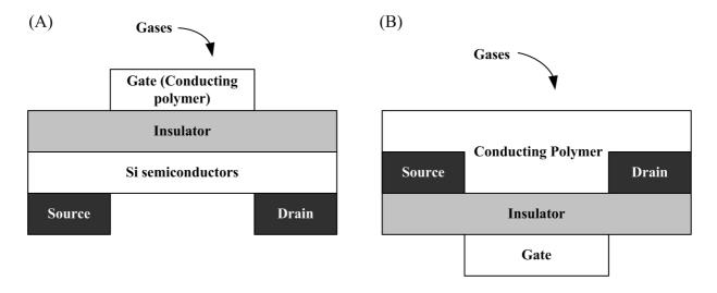
Figure 6. Configuration of TFT (A) and IGFET (B).
