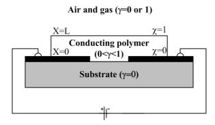
**Figure 1.** Device configuration used by Bartlett to investigate adsorption of conducting polymer films in chemresistor type sensor.
