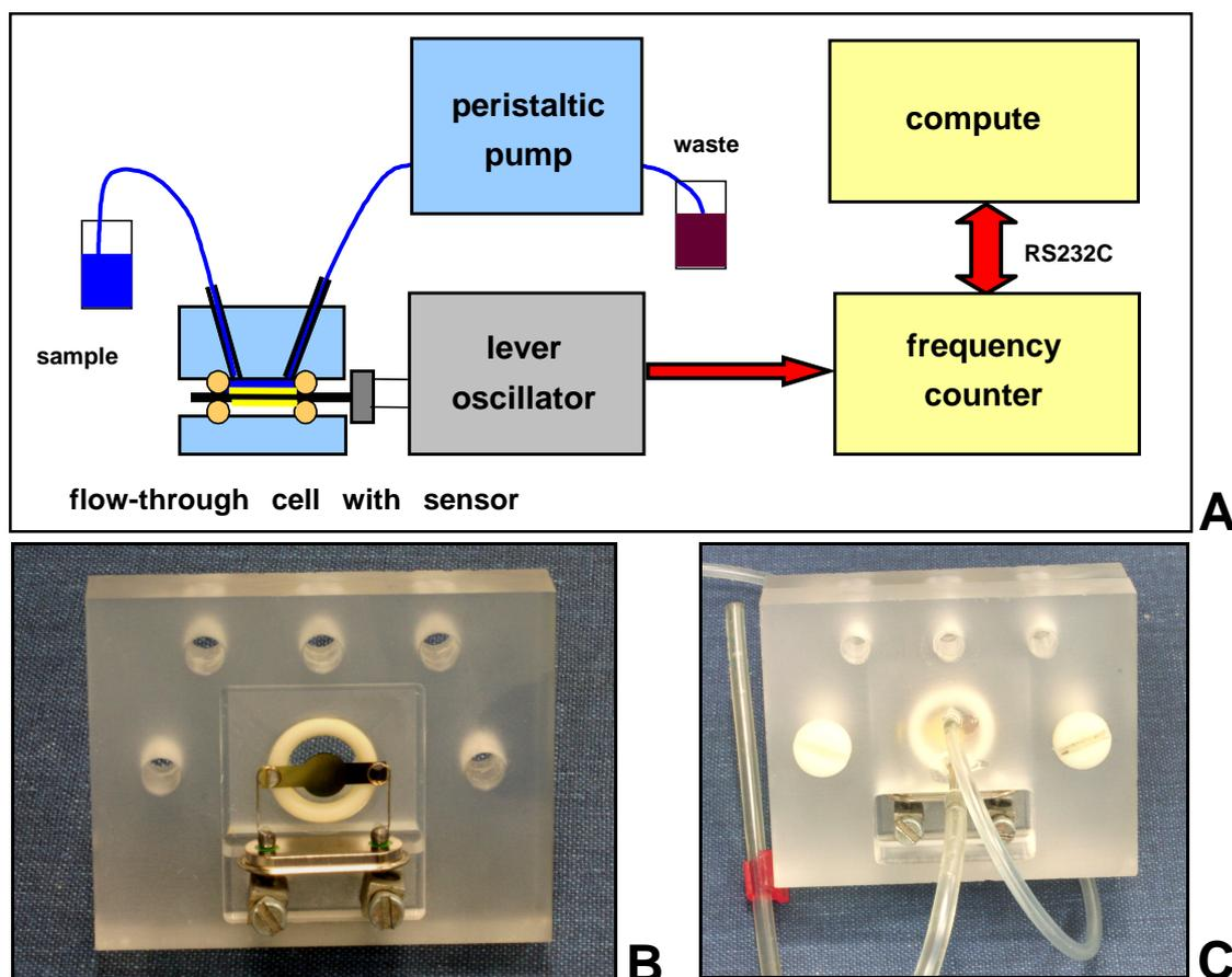
**Fig. 1.** (A) Schema of the measuring setup consisting of the flow-through cell with the piezoelectric quartz crystal; opened (B) and assembled (C) views. The sensor is driven by the lever oscillator and the output frequency is recorded using a general-purpose counter and continuously transferred to the computer. Flow is realized using the peristaltic pump.
