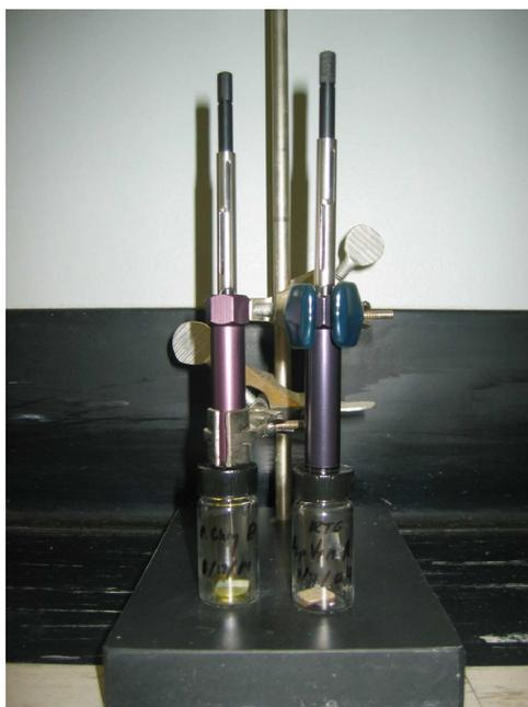
**Figure 2.** Photograph of initial Solid Phase Microextraction apparatus.
