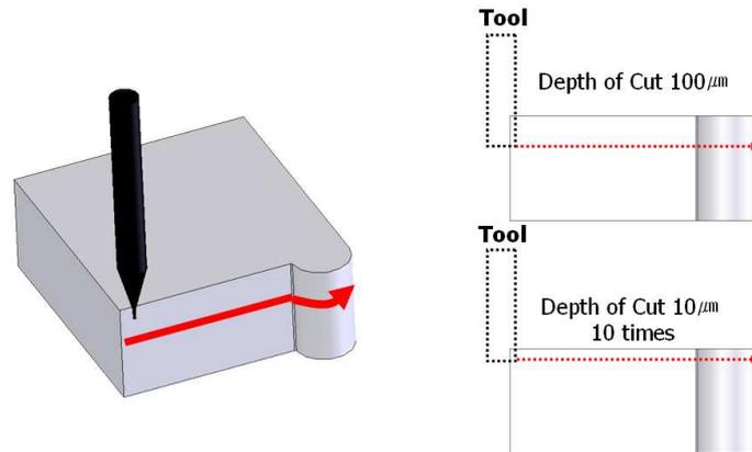
Figure 4. Cutting methods for experiments.
