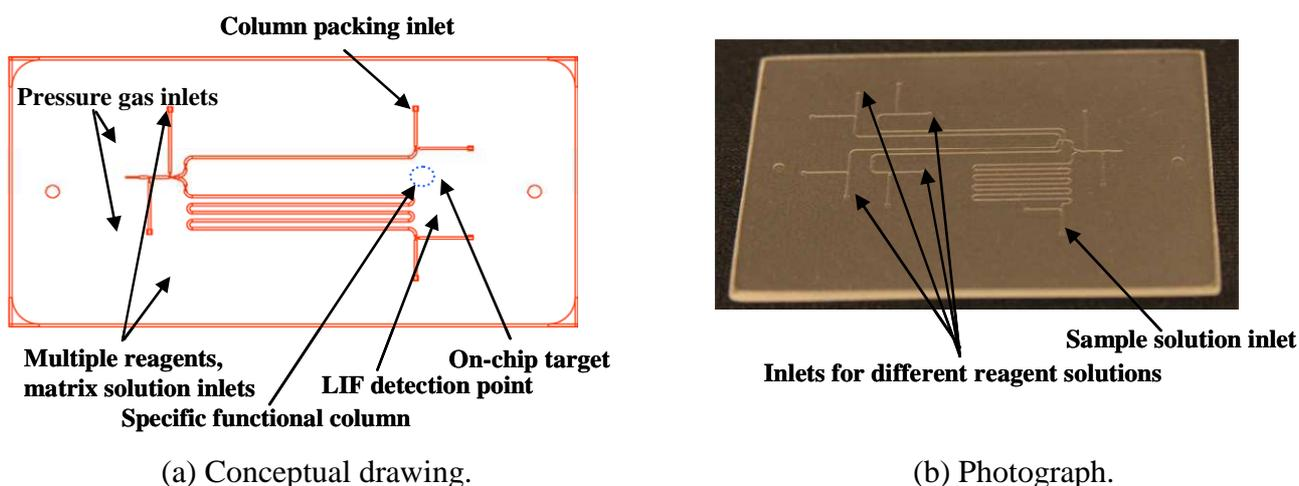
Figure 1. A disposable lab-on-a-chip device with a specific bead packed column for MALDI-MS.[3]
