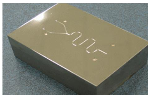
(b) Machined core by micro end-milling.
