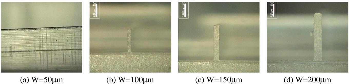
Figure 13. Test injection results using Topas8007S-04.
