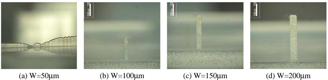
Figure 12. Test injection results using Topas5013S-04.
