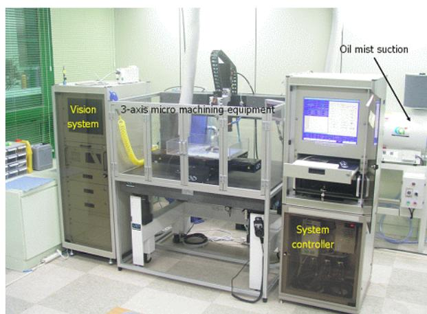
(a) 3-axis micro machining stage.
