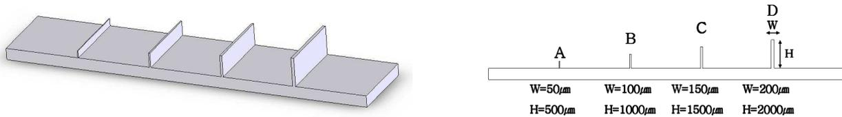
Figure 11. Micro rib feature for test injection experiments.
