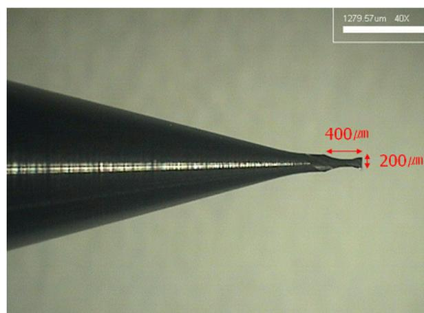
(b) Micro end-mill (diameter=200 $\mu\text{m}$ ).
