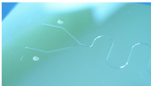
(c) Micro-fluidic channel on the core.
