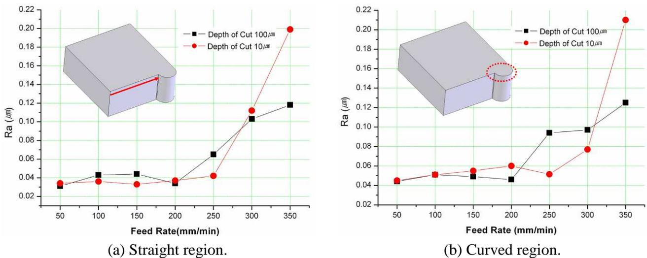
Figure 5. Measured surface roughness.
