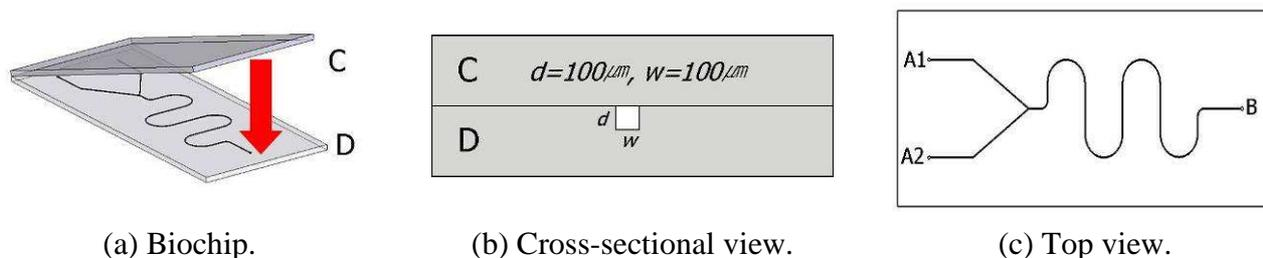
Figure 2. Designed simplified micro-fluidic channels for experiments.
