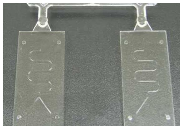
(b) Test injected biochips.
