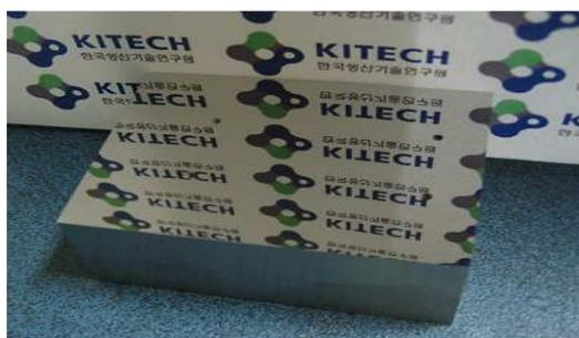
(a) Bottom plate core after mirror-finishing.
