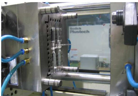
(a) Mold set for test injection.
