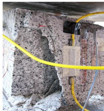
**Figure 8.** Specimen 2 after failure (Face 1 being sheared off).
