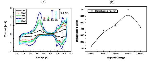
Figure 4(a) shows cyclic voltammograms in 1 mol  $L^{-1}$  sulfuric acid solution of nanoporous Pt electrodes fabricated by electroplating at various applied charges from 25 to 65 mC/mm<sup>2</sup>. In this step, the applied voltage and temperature were fixed at -0.12 V and 25 °C, respectively. The nanoporous Pt electrodes were repetitively fabricated and tested under the respective charge conditions more than five
