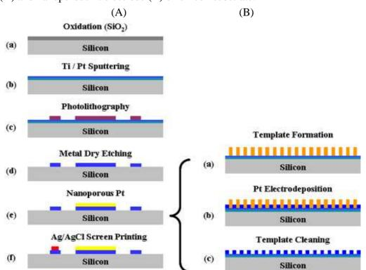
**Figure 2.** Fabrication procedures of non-enzymatic glucose micro-sensor with nanoporous Pt WE (**A**) and nanoporous Pt electrode (**B**) on silicon substrate.
