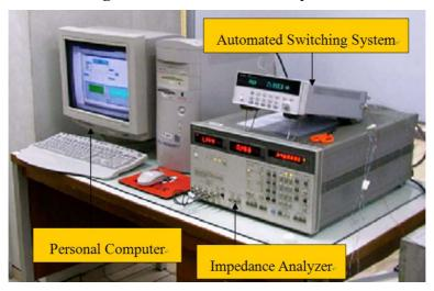
Figure 2. EMI measurement system.
